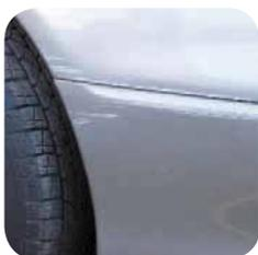
Minor dents (20mm in diameter) are acceptable as long as the paint surface has not been penetrated so that bare metal
