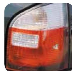
All lamps must be operational. Minor scuff marks or scratches are acceptable, but holes or cracks in the
