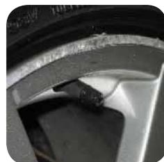
Dents or damage to the rim or main body of the wheels are not acceptable. All four wheel trims must be intact,
